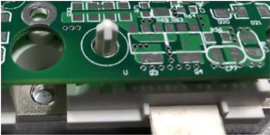
Figure 9: Align PCB to the power module.
